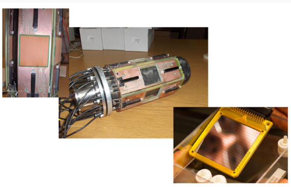
Figure 1. Comparison between the old and new setups. The previous setup (a) used 5 telescopes, each with a MWPC to gather the position of the particles and a thin scintillator in front of the main one to differentiate the particles and positrons from gammas. The new setup (b) consisted of 6 telescopes, and the MWPCs was replaced by DSSDs, which can be used for the particle identification, removing the need for the thin scintillators.
