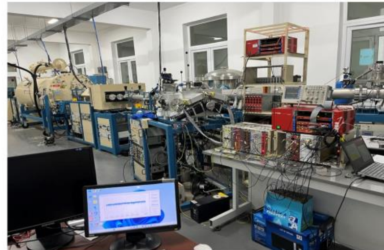
Picture in lab of the detector system and the DAQ connected to Pelletron
