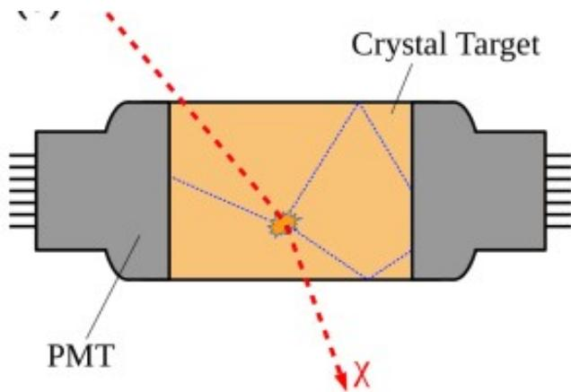
Cryogenic bolometer (with charge or light readout)
